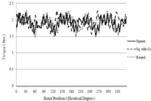
Fig 2: Torque profile comparison for different types of slot designs for 200 W, 24 Volt, 1000 rpm Motor
