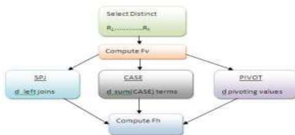
Fig. 3 shows steps on all methods based on table containing results of vertical aggregations
