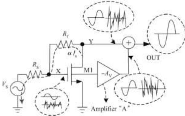
Fig2. Wide-band LNA exploiting noise-cancelling technique.
