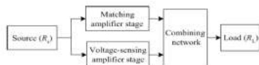
Fig1. Wideband gain-flattened LNA architecture.
