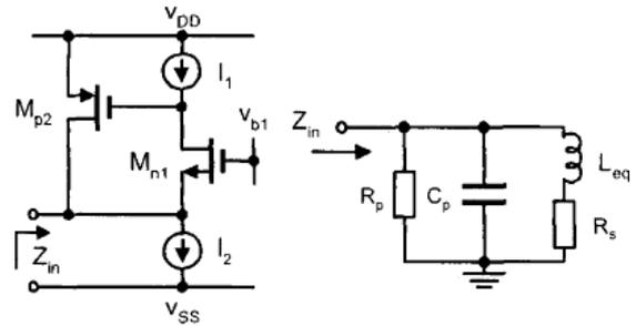
Fig3. A novel RF CMOS grounded active inductor and its small-signal equivalent circuit model.
