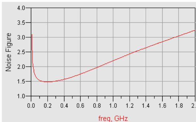
Fig7. Noise figure of simulated LNA.
