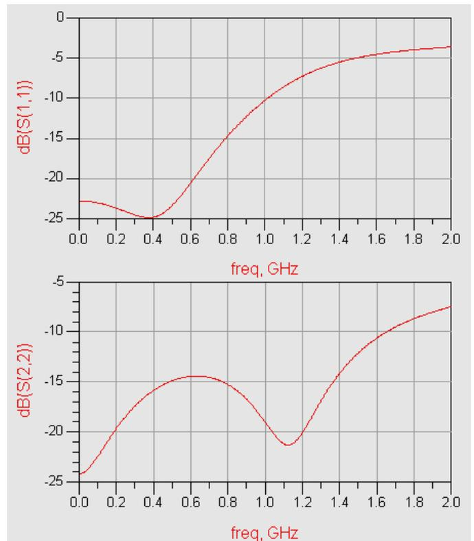
Fig. 9..Input and output matching diagram.
