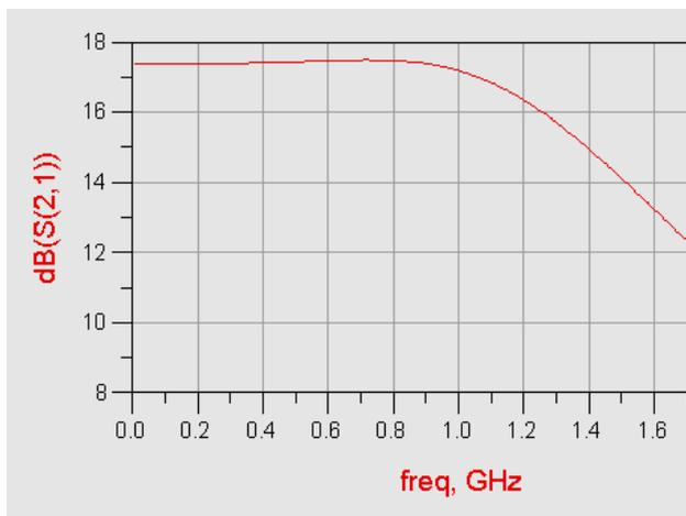
Fig 8.Gain of simulated LNA
