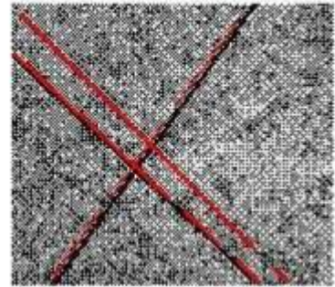
Fig. 7 Edge detection results for noisy image using Hough Transform
