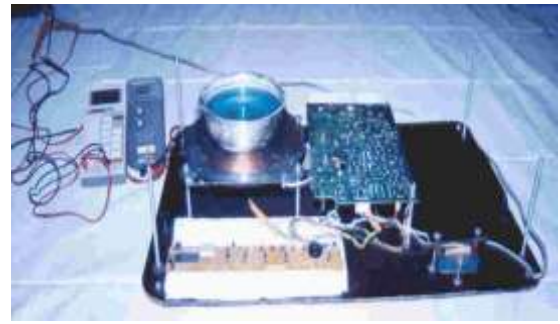
Fig. 10 Assembly of one cooking zones out of two zones
