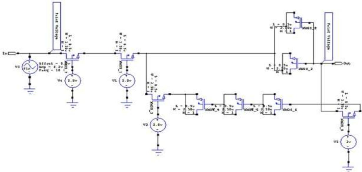
Fig. 2.(b): Realisation of amino acid (Alanine) Model using active MOS Component
