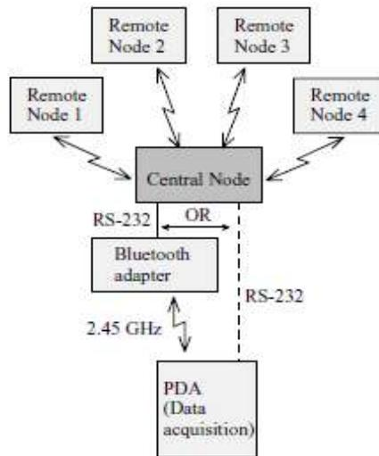
Fig2–The general network topology used in WBAN
